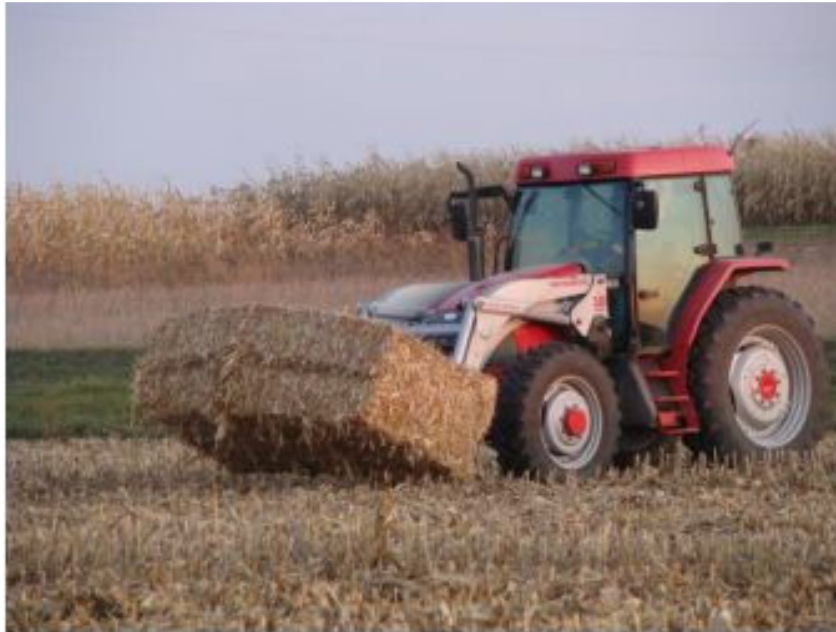
Figure 4: Tractor mounted bale spear used to maneuver bales of corn stover at the edge of a field.
