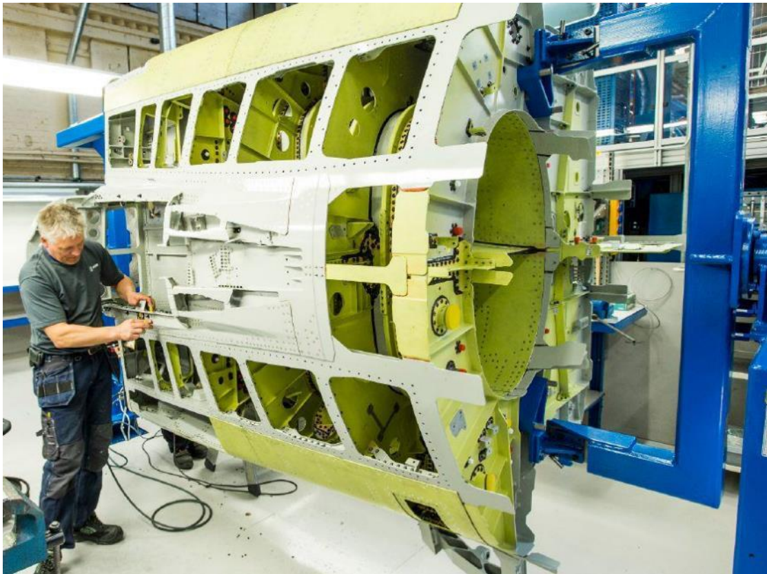
Figure 18. Part of Gripen divided by ribs (Kustvik, saabgroup.com, 2016).
