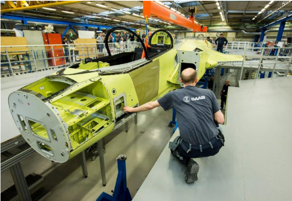
Figure 16. Gripen is positioned into a fixture (Kustvik, saabgroup.com, 2016).
